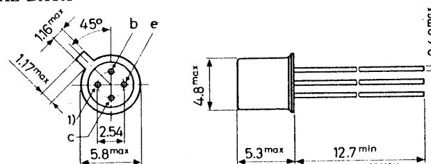
1) = shield lead (connected to case)
