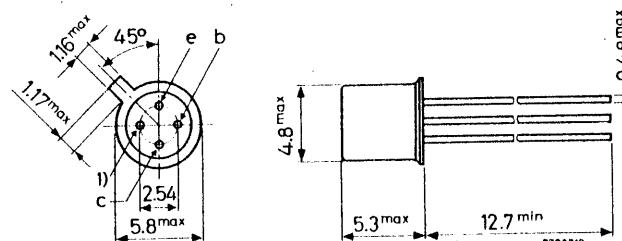
1) = shield lead (connected to case)
