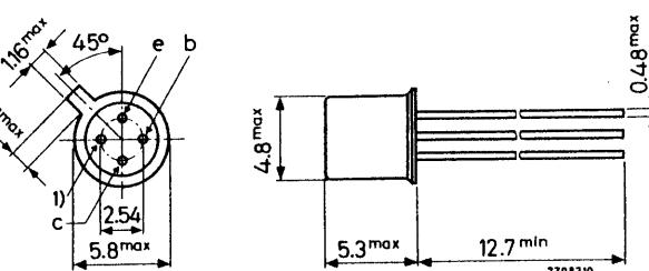
1) = shield lead (connected to case)
