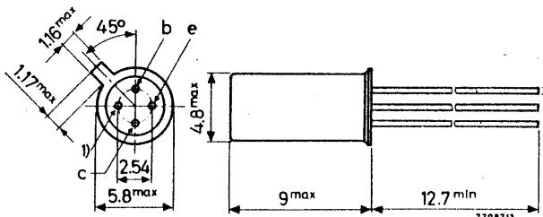
! = shield lead (connected to case)
