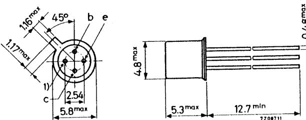
1) = shield lead (connected to case)
