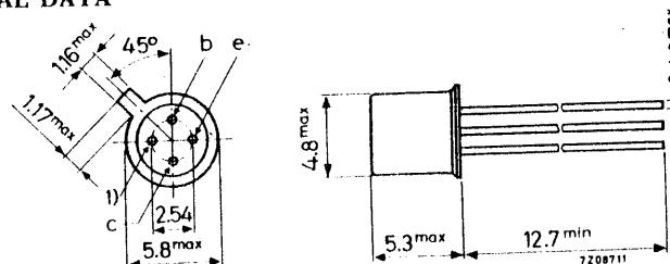
1) = shield lead (connected to case)
