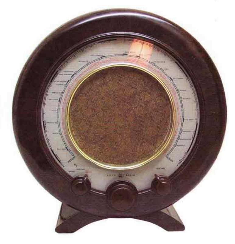
restuffed with modern components and refitted at this time also. At least the set now had a consistent type of capacitor and resistor fitted of the correct values and in my opinion looked much better for it even if a little more of the remaining originality had been lost by doing so.
