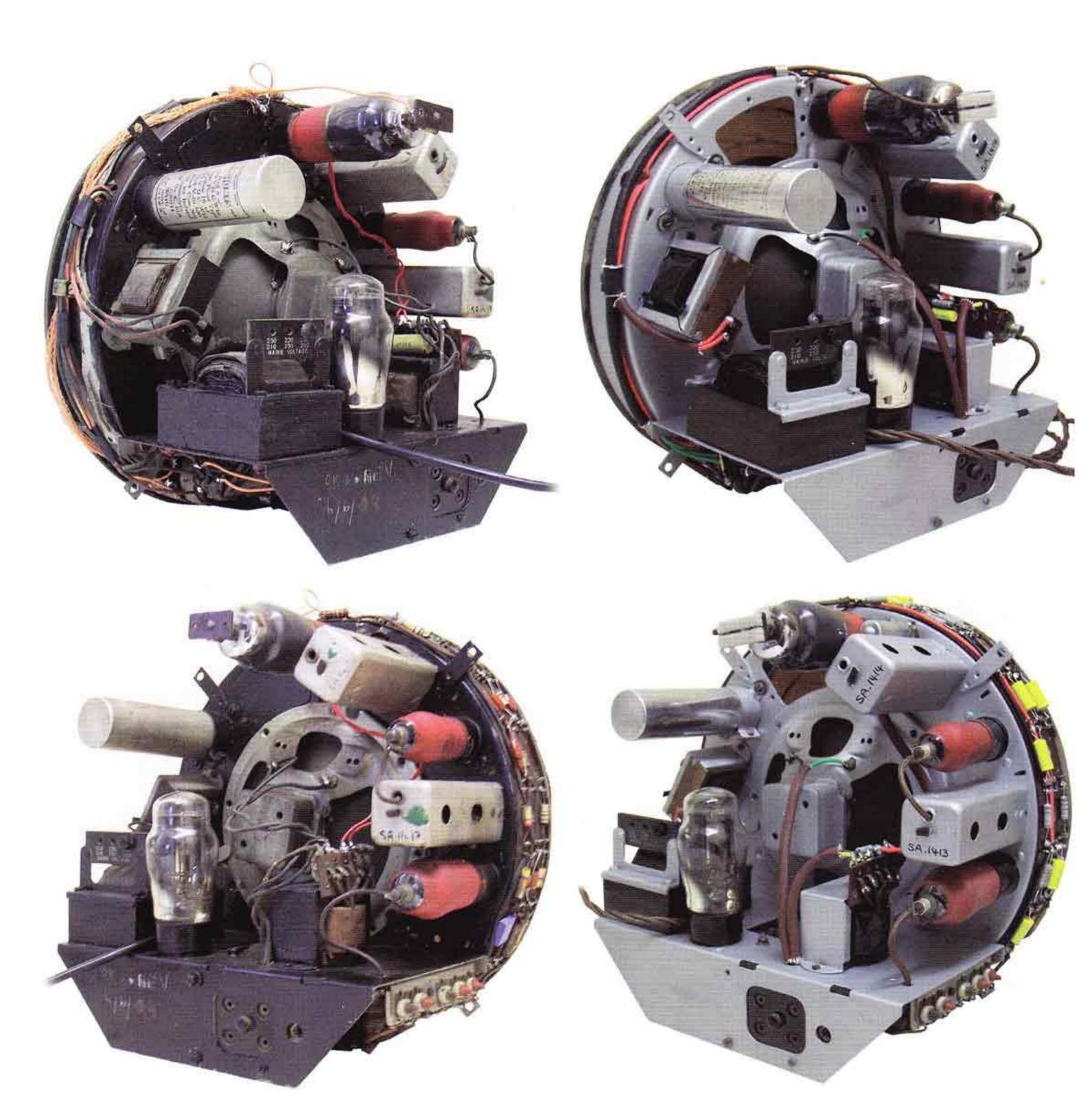
apparently whatever type and value was to hand at the time. Some of the resistors had been changed as well, again seemingly with whatever was to hand. But the 'new' wiring really was something! Most obvious a crude screening braid made from what I assume was the outer layer of a piece of co-axial cable. I'll leave the 'before' and 'after' images to illustrate in detail and speak for themselves here.
