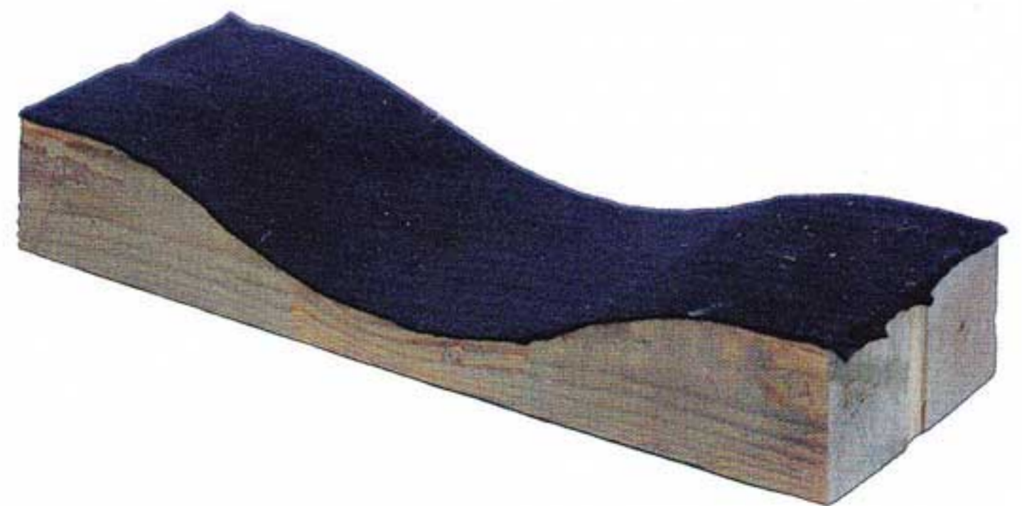
Below: Former to help veneer keep shape on curved top of Philips set
