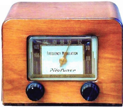
Figure 9 (above): Front view of the 1947 Pilotuner T-601, typical of an FM-only tuner capable of being plugged into the 'gram' input of an existing AM radio.
