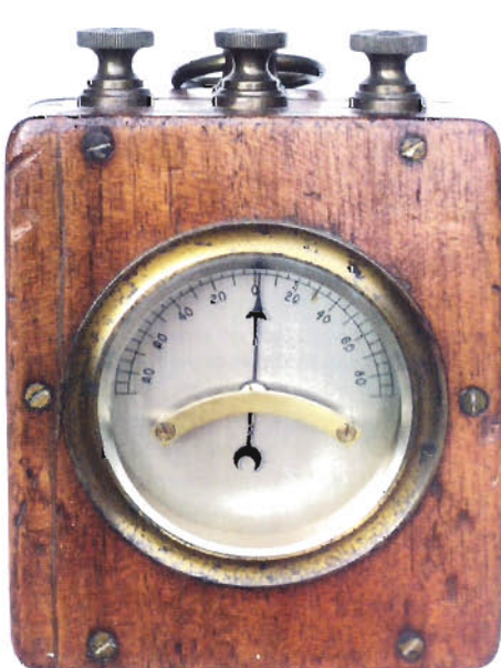
Fig 5: Linesman's Galvos (a&b) unnamed. (c) WG Pye & Co 1917
