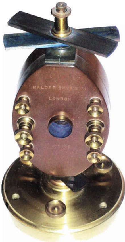
Fig 4a: Astatic Tangent Galvanometer (Nalder Bros) inertia when it is a rotary motion) should be as small as possible which is why meter pointers are frequently made from thin aluminium tubing. If, however, the size of the moving magnet or coil is reduced this will tend to reduce the sensitivity of the instrument. Stiffness can also be increased to speed up the response but this again reduces sensitivity. The equation used to calculate the frequency of a tuned circuit ( f_0 = 1/2\pi(LC)^{1/2} ) can be used by substituting mass or moment of inertia divided by stiffness (m/S) for (LC). The response times of galvanometers and pendulums are sometimes given for a swing in one direction rather than the full period T = 1/f_0 .
