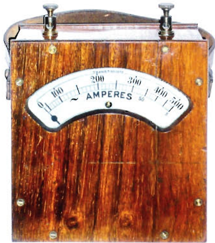
Fig 15: NCS Spring-controlled ammeter (repulsion)
