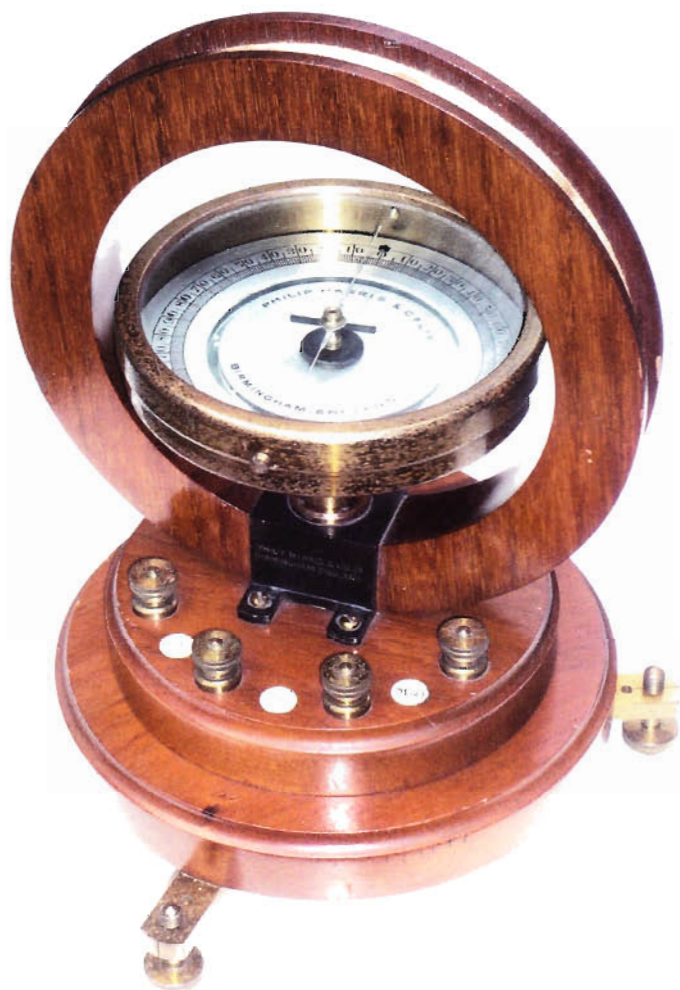
Fig 1: Tangent Galvanometer (Philip Harris & Co Ltd)
