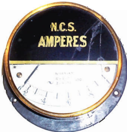
Fig 14a: NCS Gravity Ammeter (repulsion)
