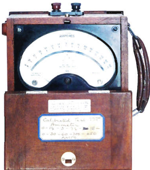
Fig 21a: Sub-Standard Ammeter (Everett Edgcombe)
