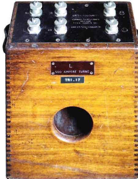
Fig 16: Current Transformers (a) Smith Hobson Ltd.
