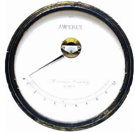
Fig 13a: Rummy & Rummy Ammeter (repulsion)
