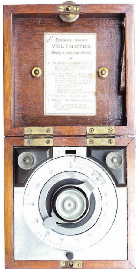
Figure 18. Fleming & Gimingham electrodynamic type
