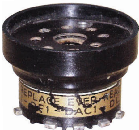
Figure 7: The Octal-to-Ct8 adaptor, made by Ever Ready. On the adaptor it says 'Only to replace Ever Ready valves DK1 - DF1 - DAC1 - DL2'
