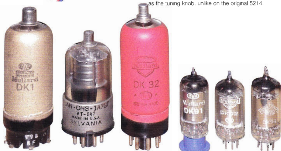
Figure 12: Line-up of 1.4V frequency changer valves. Left-to-right are: DK1, 1A7GT (VT-147), DK32, DK91, DK92 and DK96. Mullard has supplied the DK91 with a plastic cover for the pins, helping prevent them from being bent during handling. The DK96 is marked 'Ever Ready', but as with earlier Ever Ready valves, this was manufactured by Mullard.
