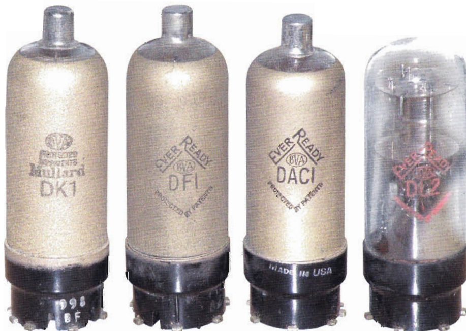
Figure 4. An 'identity parade' line-up of the DK1, DF1, DAC1 and DL2 valves from my Ever Ready 5214.
