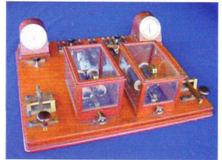
13: A repeater station
